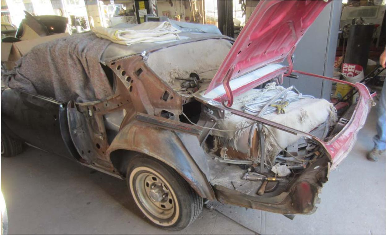
the doors needed rebuilding at the bottoms and the corners as well as new sheetmetal “skins”, the front fenders contained hundreds of rust pin-holes that had been puttied over and painted, there was a 3” diameter hole in the roof near the driver’s A-pillar – also puttied and painted. It
