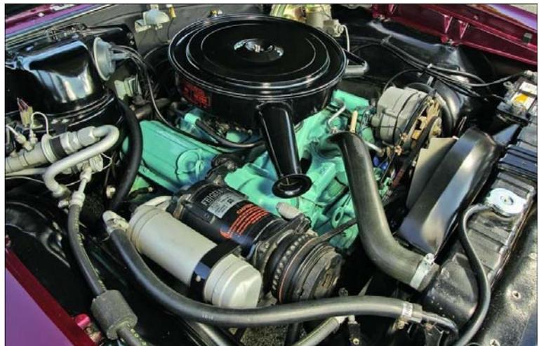
**The original 326 H.O. V-8 Engine was bored .030 over and upgraded with a longer-duration camshaft and a 650-CFM carb during its rebuild**
