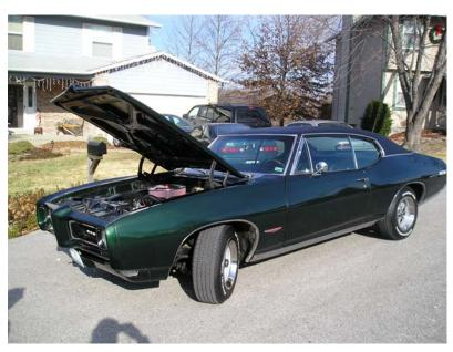
This past winter and spring some modifications were made under the hood and to the rear of the car. My mechanic, Randy Bardle, found a 428 engine he thought I needed. Between Randy and Bob Stiegemeier, the 428 was reworked with forged pistons, roller rockers, different heads and a Ram Air exhaust manifold. A MSD electric system was installed along with a Stiegemeier racing carb
